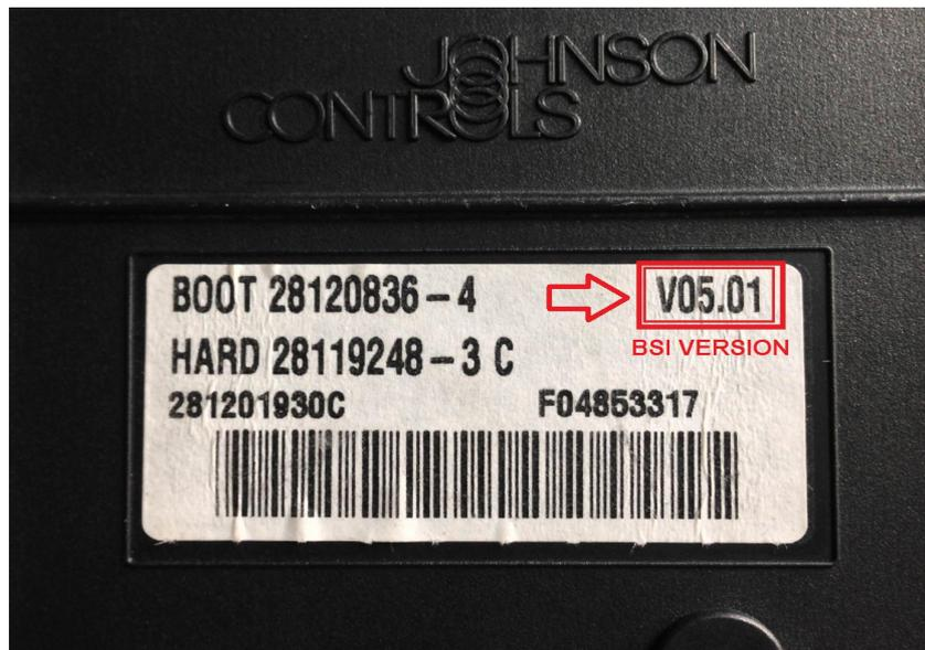
The BSI from the picture is V5.01 and can be found in vehicles from 2008 to now. The older vehicles have HW version V2.00 and are typical from 2004 to 2008.
