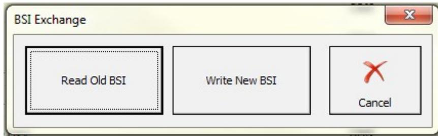
This dialog allows you to read the whole content of the one BSI (JCI or Valeo CAN) and transfer it to the new one. It is very important to use the same hardware type of the replacement BSI. The Valeo BSIs are two types - the old one is thick, while the new one is thin, so they can't be mistaken. The JCI BSIs are also two types, but they can't be identified by their exterior, because both are thin. In this case take a look at the sticker for a HW version
